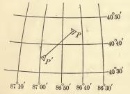
drawn on the polyconic projec-40°50' tion method which is explained in Art. 69. Station *P* is located at latitude 40° 45' and at longitude 86° 43', while station *P'* is located at latitude 40° 36' and longitude 86° 58'. The straight line, or geodesic, joining the
